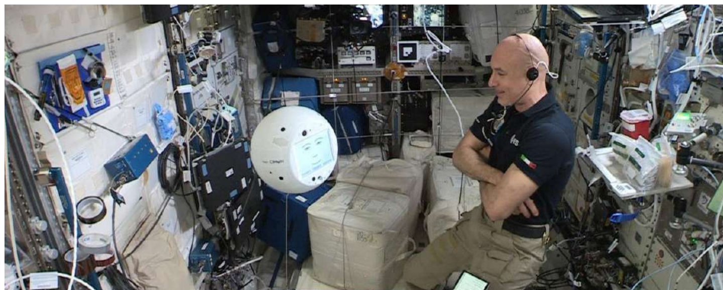
In February 2020, the upgraded version of the mobile robot assistant CIMON-2—developed in Germany—successfully premiered with ESA-Astronaut Luca Parmitano on the ISS. Image Credit: ESA/DLR/NASA
